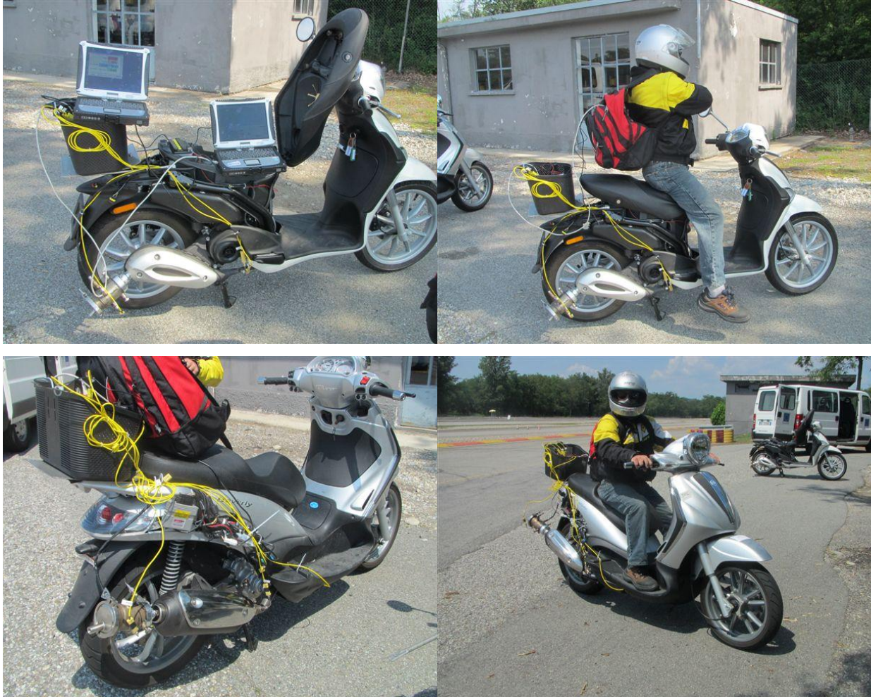
Figure 16-97: Installation of the monitoring and recording instruments on the tested vehicles
